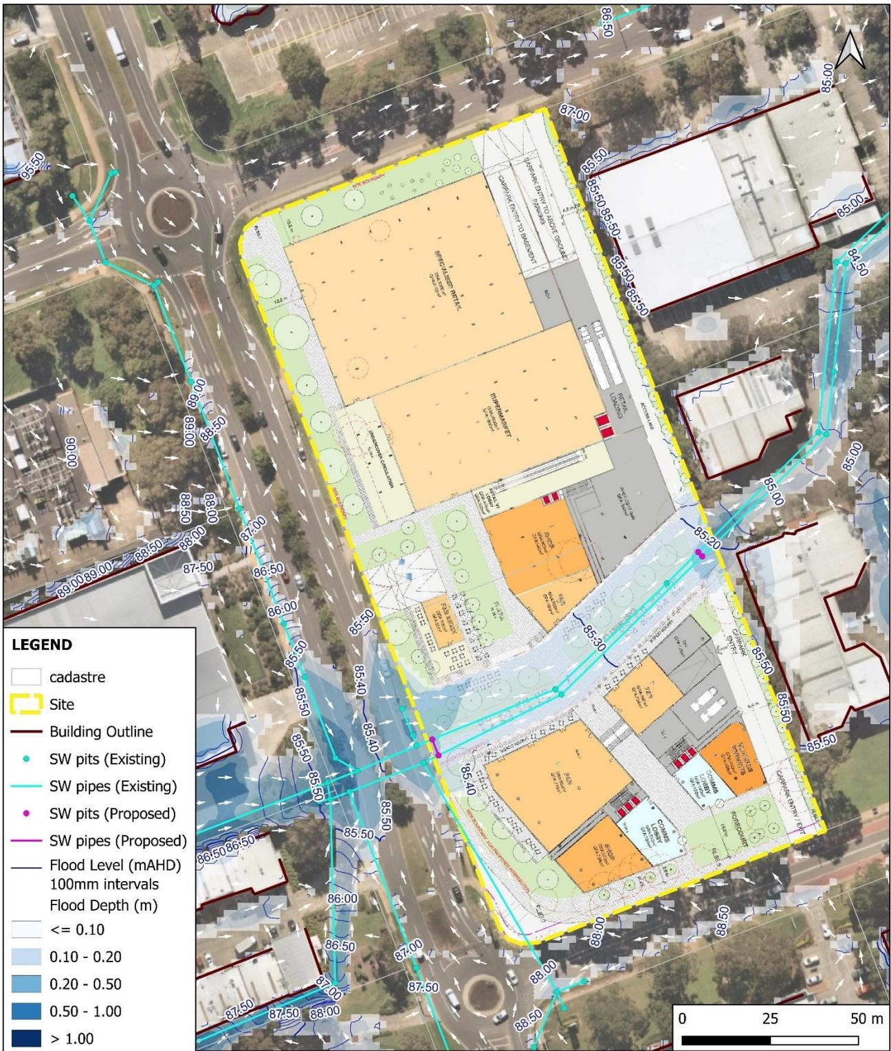
Figure 24 – Flood Levels & Depths (0.2% AEP) – Post Development Conditions (no blockage through car park) – 2013 Tuflow Engine
