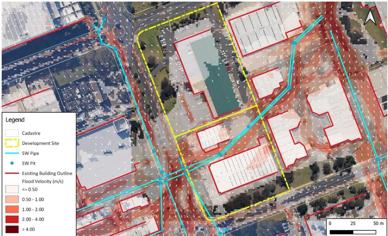
Figure 17 – Flood Velocity (PMF) – Updated Existing Conditions
