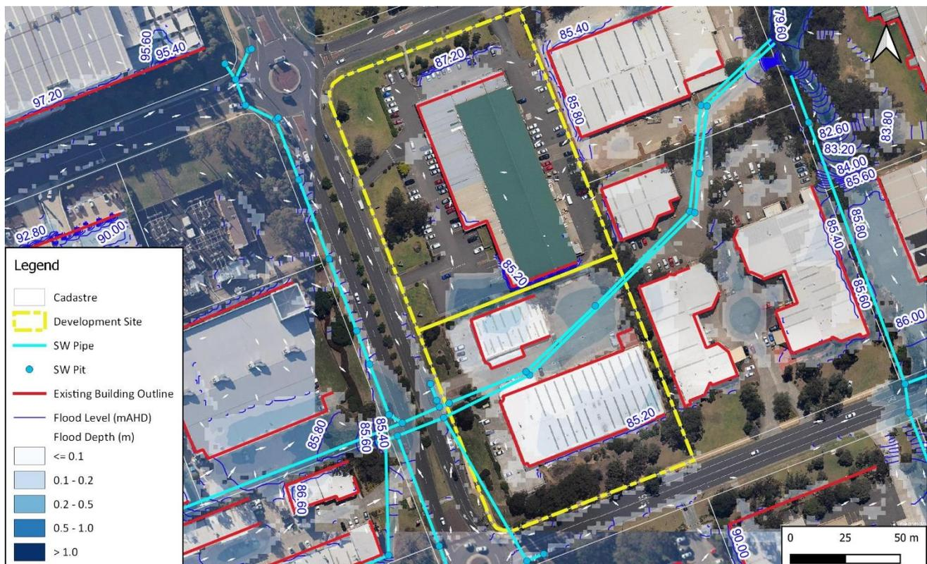
Figure 13 – Flood Level & Depth (1%AEP) – Updated Existing Conditions
