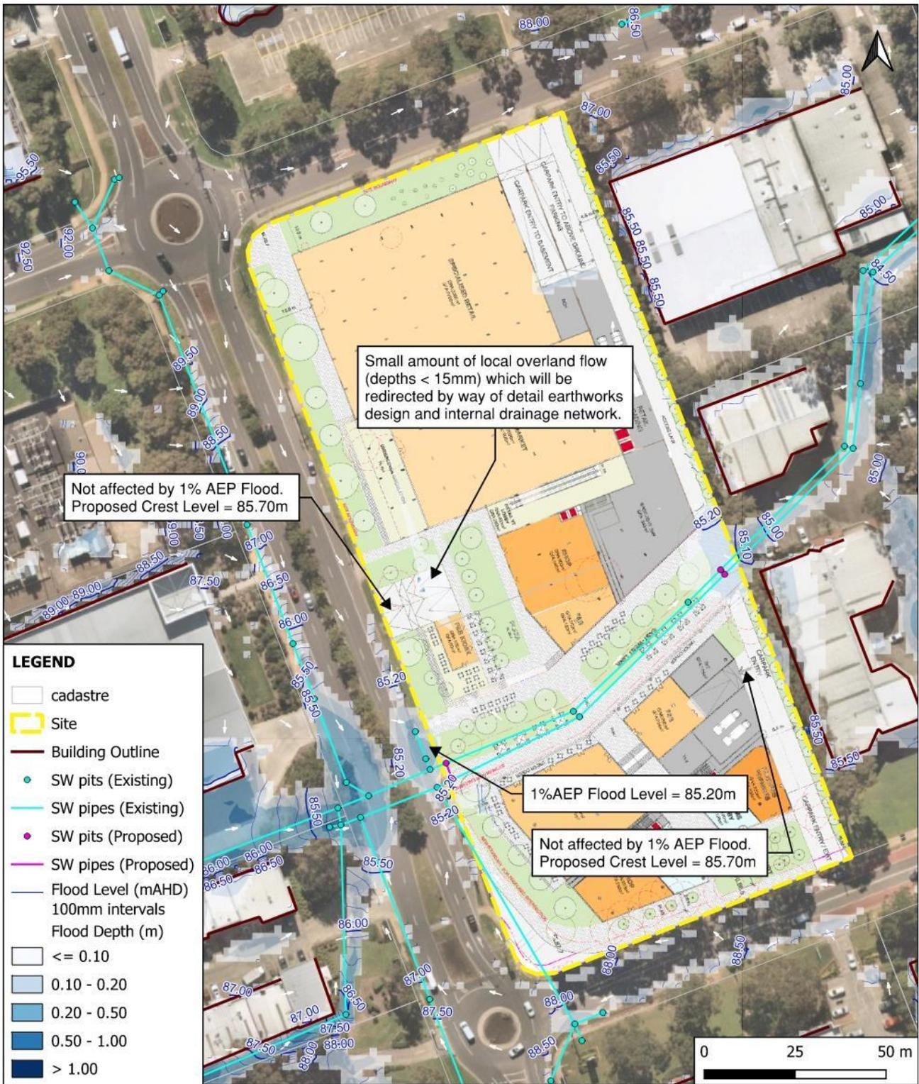
Figure 21 – Flood Levels & Depths (1%AEP) – Post Development Conditions – 2013 Tuflow Engine
