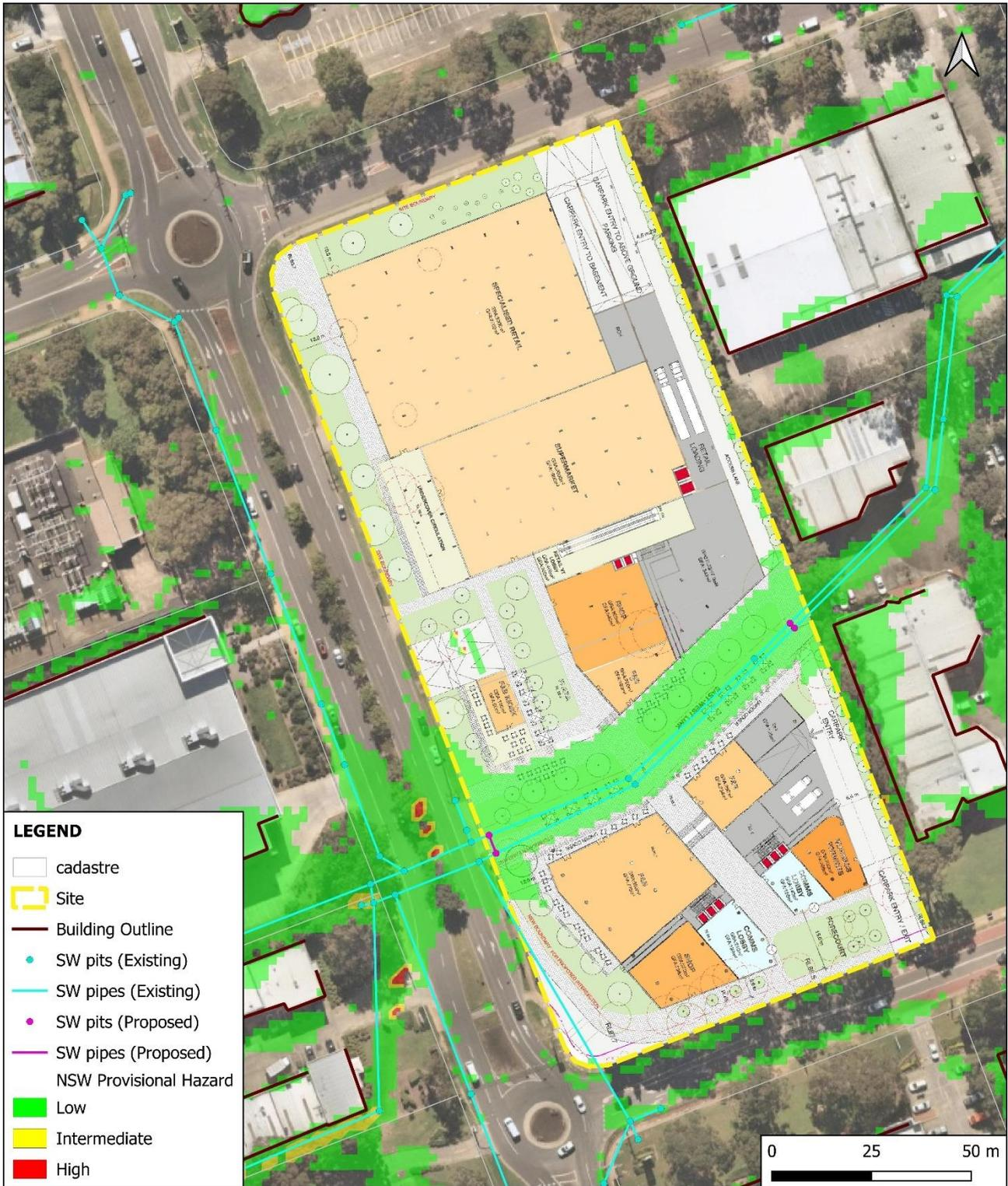
Figure 26 – NSW Provisional Flood Hazard (0.2% AEP) – Post Development Conditions (no blockage through car park) – 2013 Tuflow Engine
