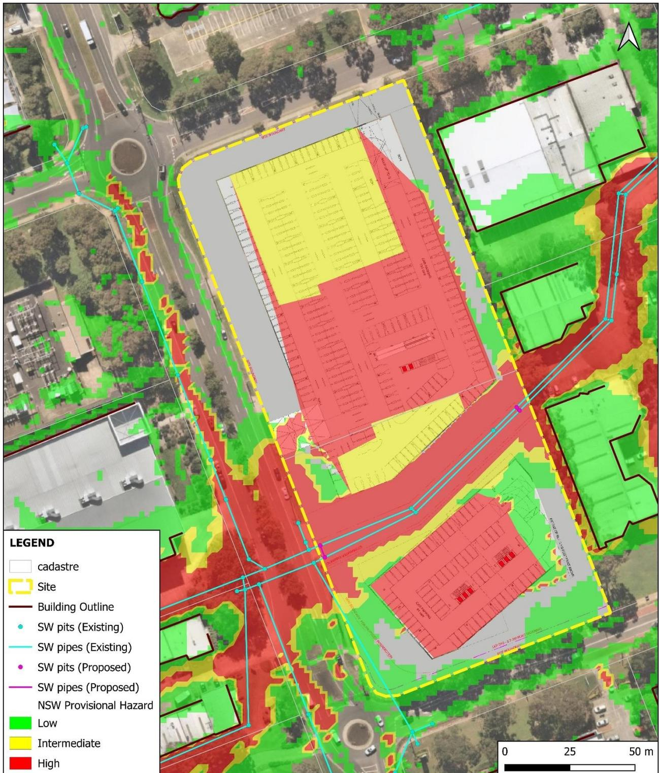
Figure 29 – NSW Provisional Flood Hazard (PMF) – Post Development Conditions (no blockage through car park) – 2013 Tuflow Engine
