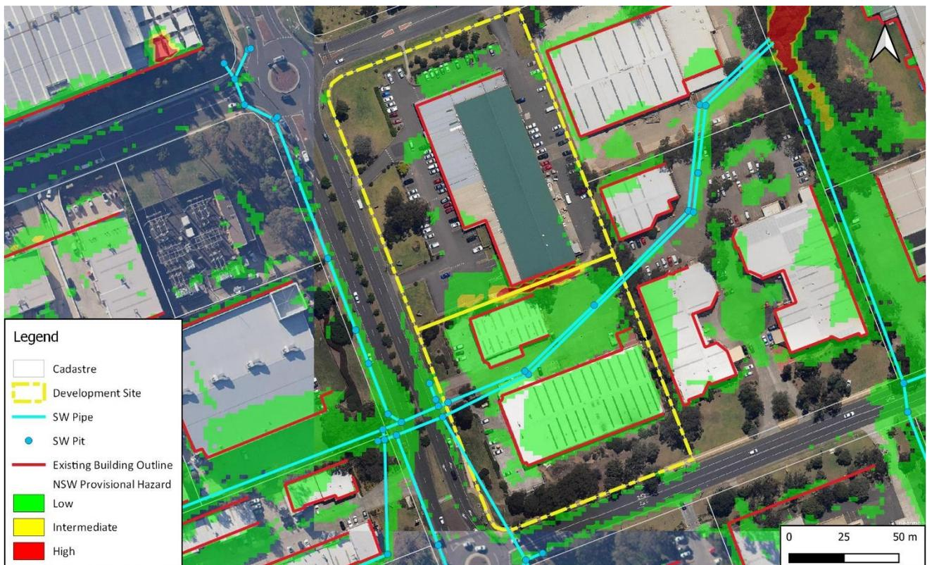
Figure 15 – Flood Hazard (1%AEP) – Updated Existing Conditions
