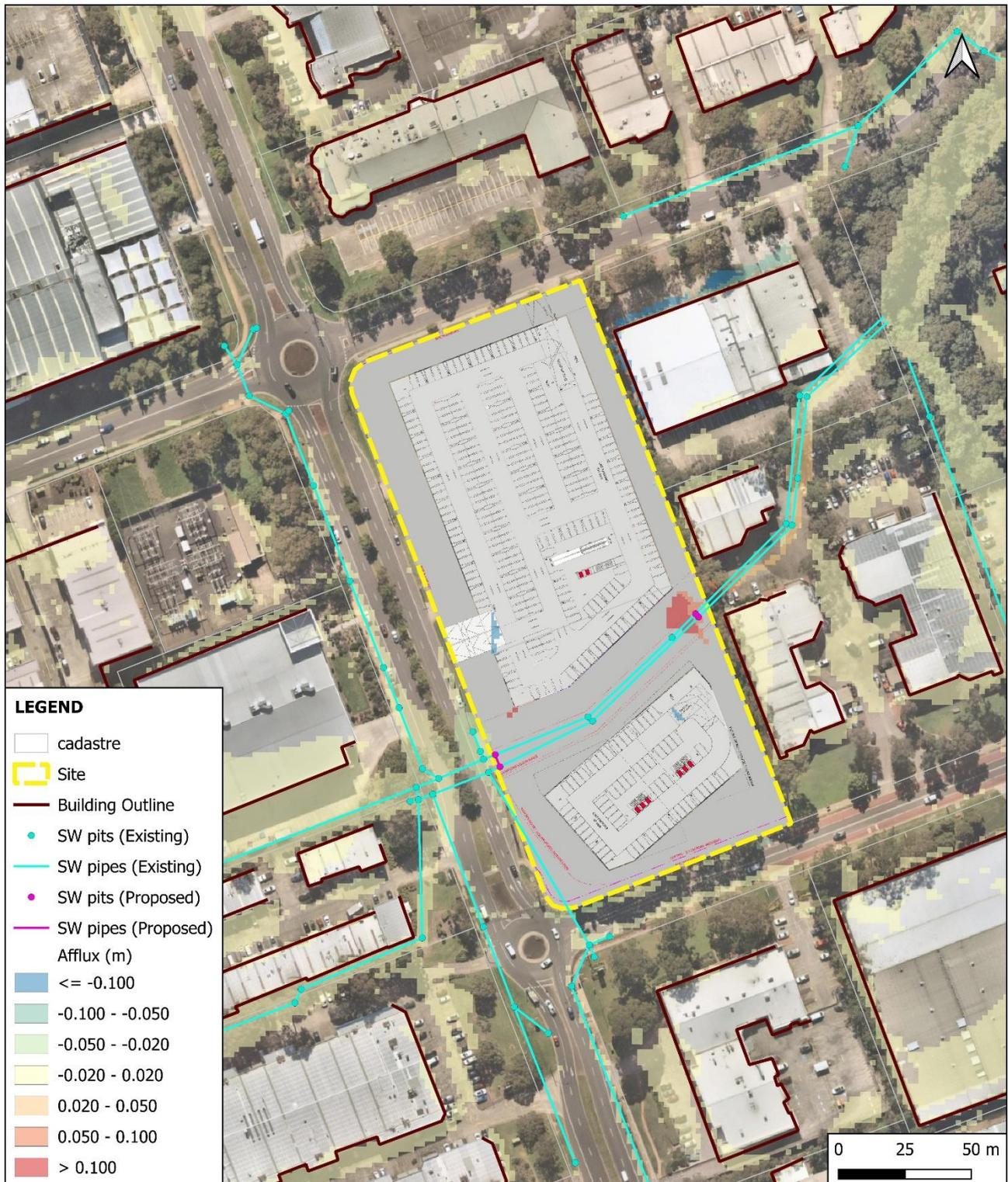
Figure 30 – 1%AEP Flood Level Impact
