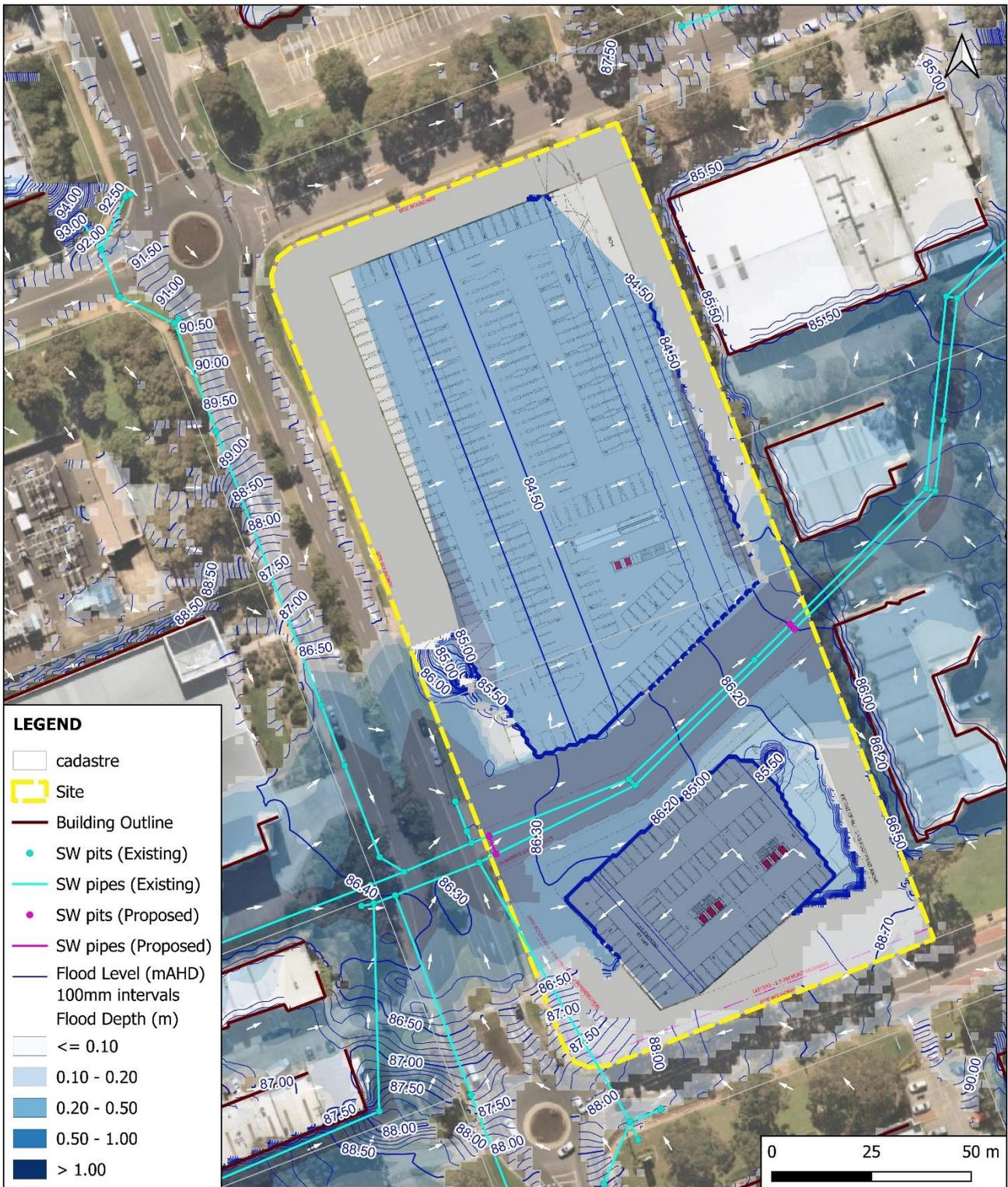
Figure 27 – Flood Levels & Depths (PMF) – Post Development Conditions (no blockage through car park) – 2013 TufLOW Engine
