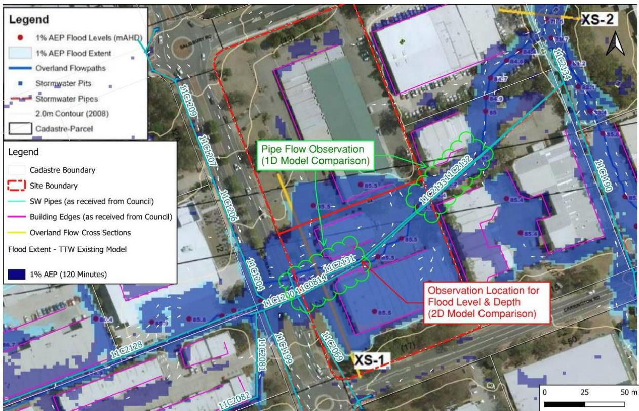
Figure 7 – Flood Comparison locations (1D & 2D) – Overlaid Council's Flood Map Received on 28/11/2021
