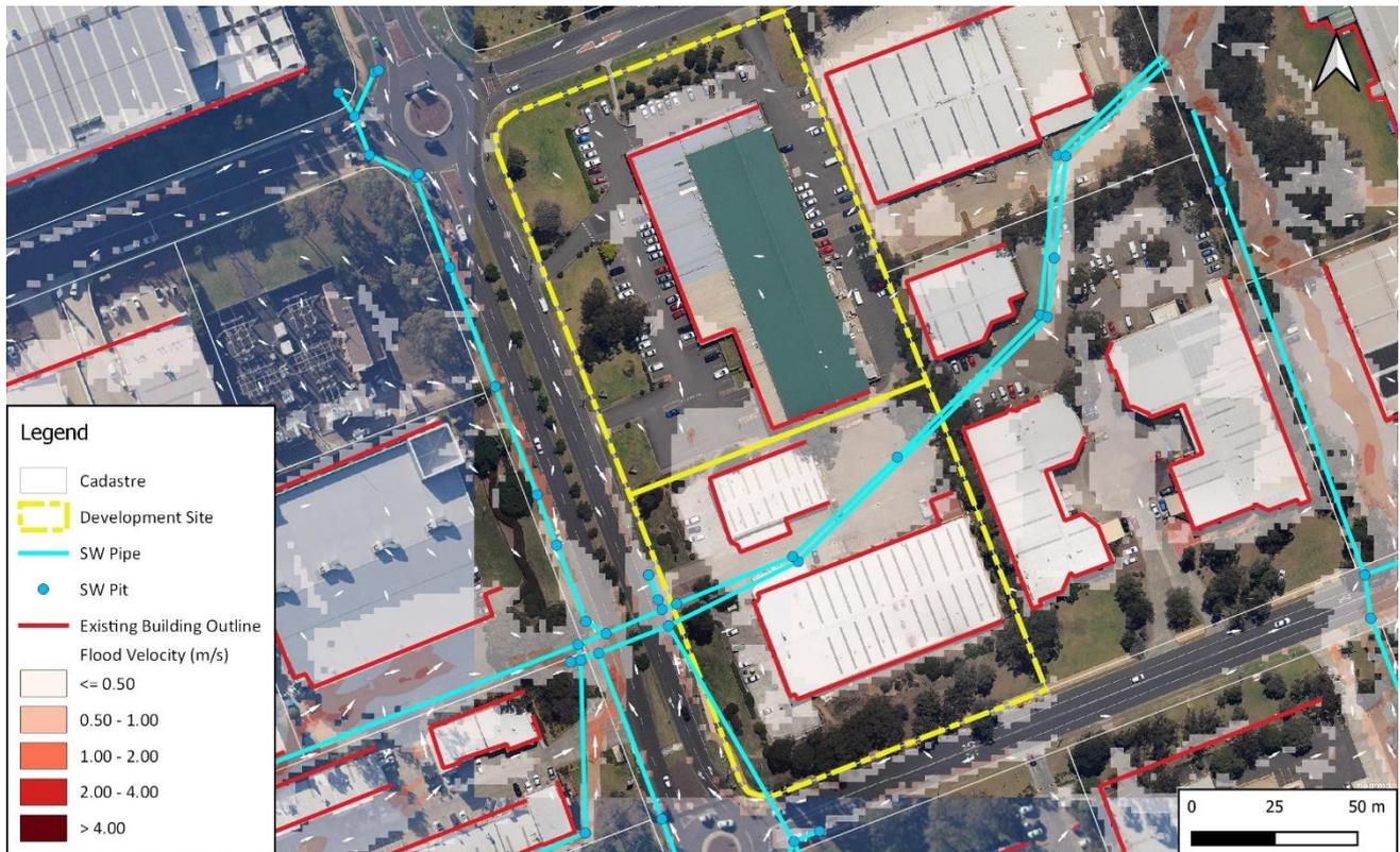
Figure 14 – Flood Velocity (1%AEP) – Updated Existing Conditions
