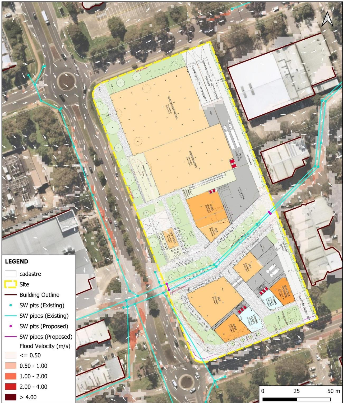
Figure 22 – Flood Velocity (1%AEP) – Post Development Conditions – 2013 Tuflow Engine
