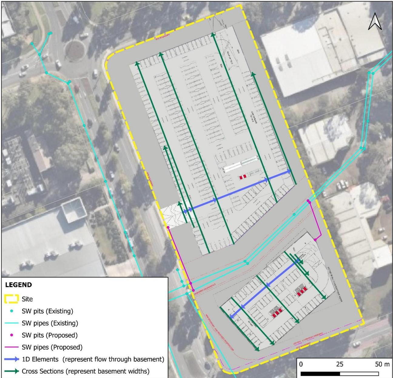
Figure 19 – Proposed Inlet Pit Locations Connected to Existing twin DN1800 Pipes
