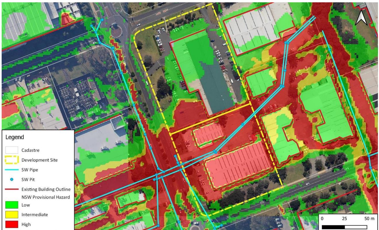
Figure 18 – Flood Hazards (PMF) – Updated Existing Conditions
