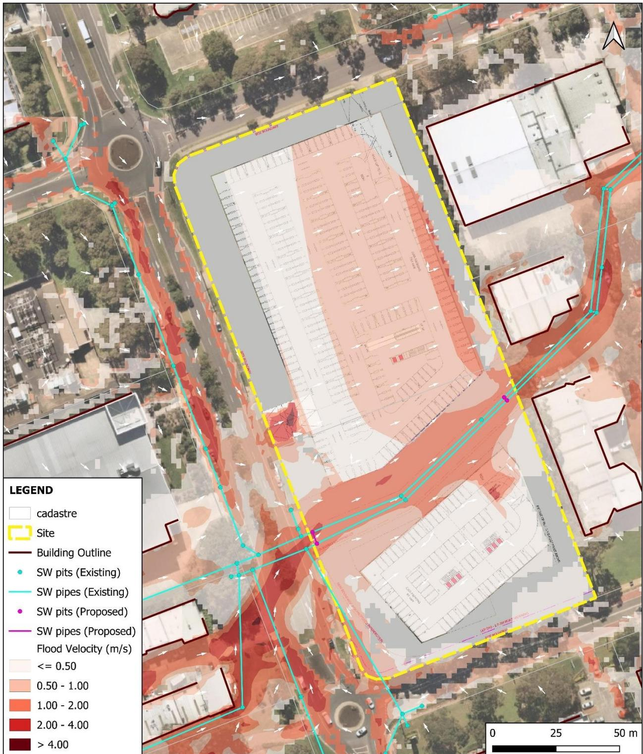
Figure 28 – Flood Velocity (PMF) – Post Development Conditions (no blockage through car park) – 2013 Tuflow Engine
