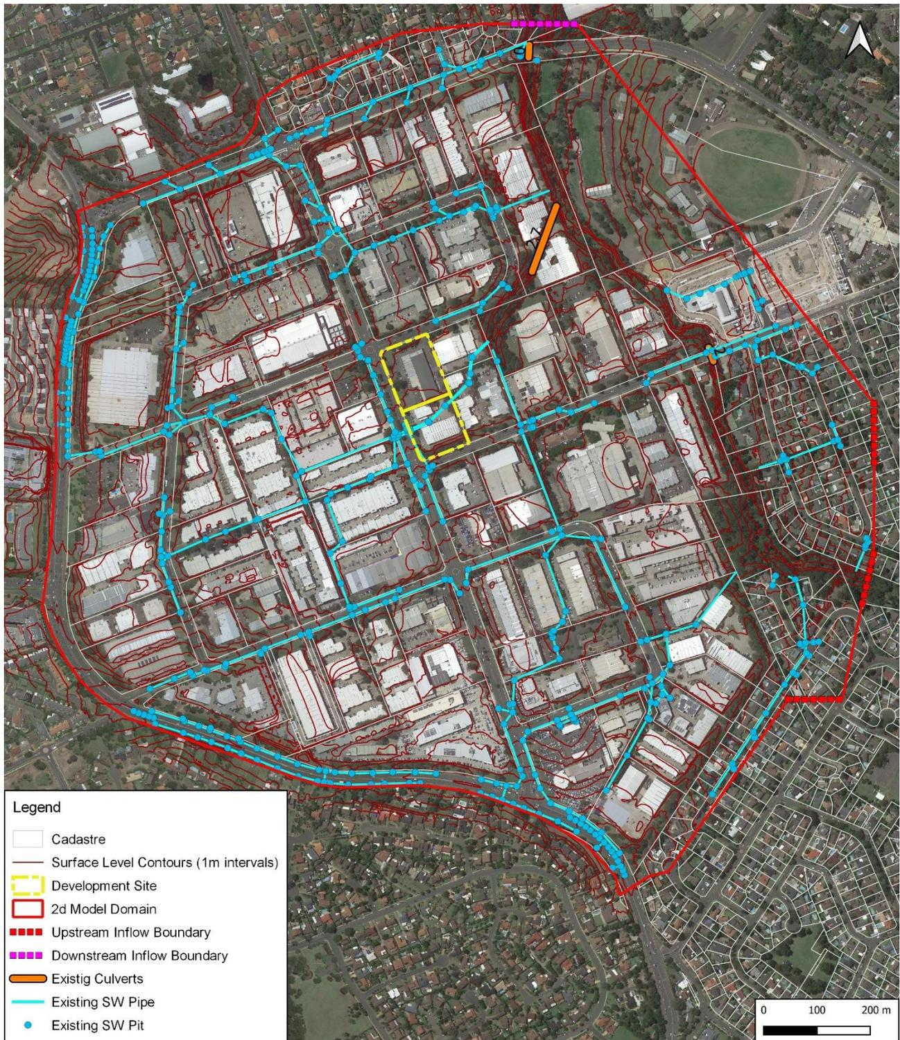
Figure 5 – TUFLOW 1d / 2d Model Domain
