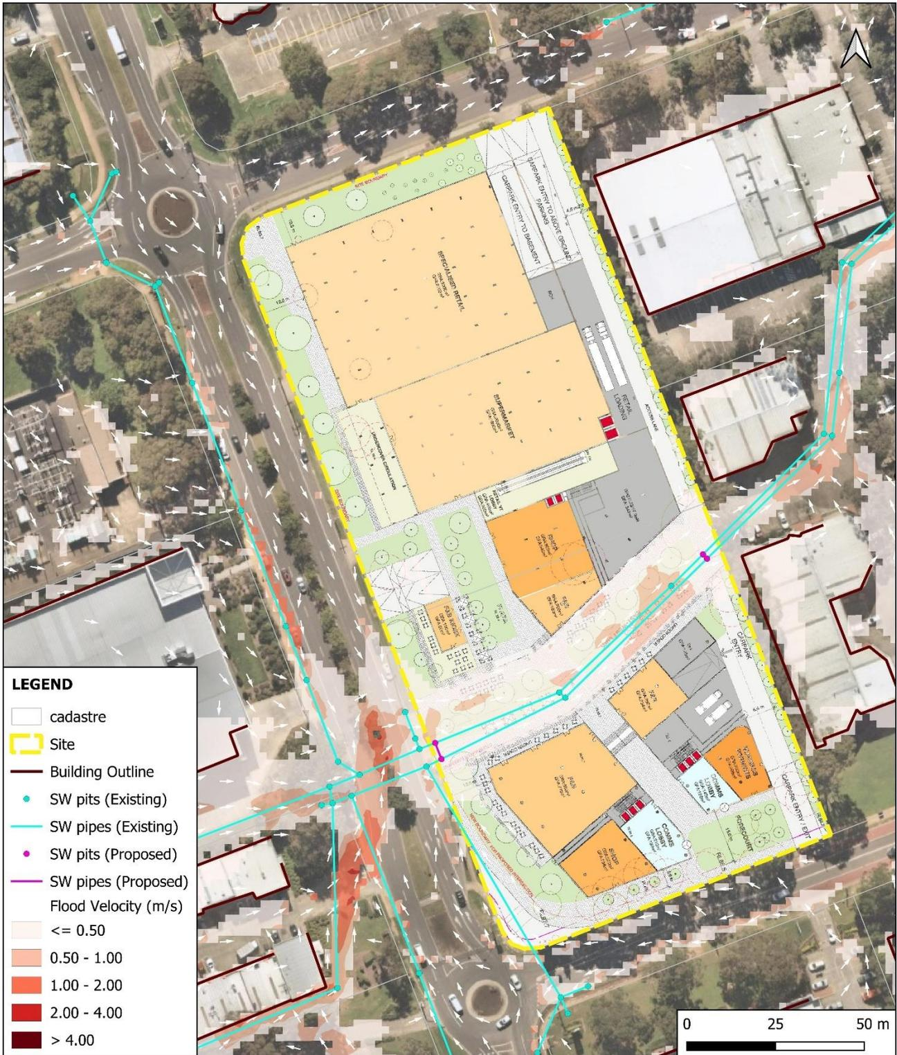
Figure 25 – Flood Velocity (0.2% AEP) – Post Development Conditions (no blockage through car park) – 2013 Tuflow Engine
