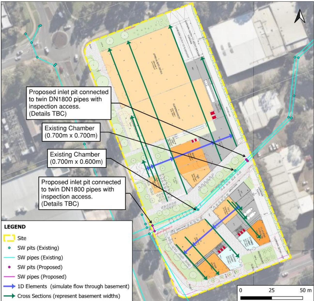
Figure 20 – Proposed Inlet Pit Locations Connected to Existing twin DN1800 Pipes
