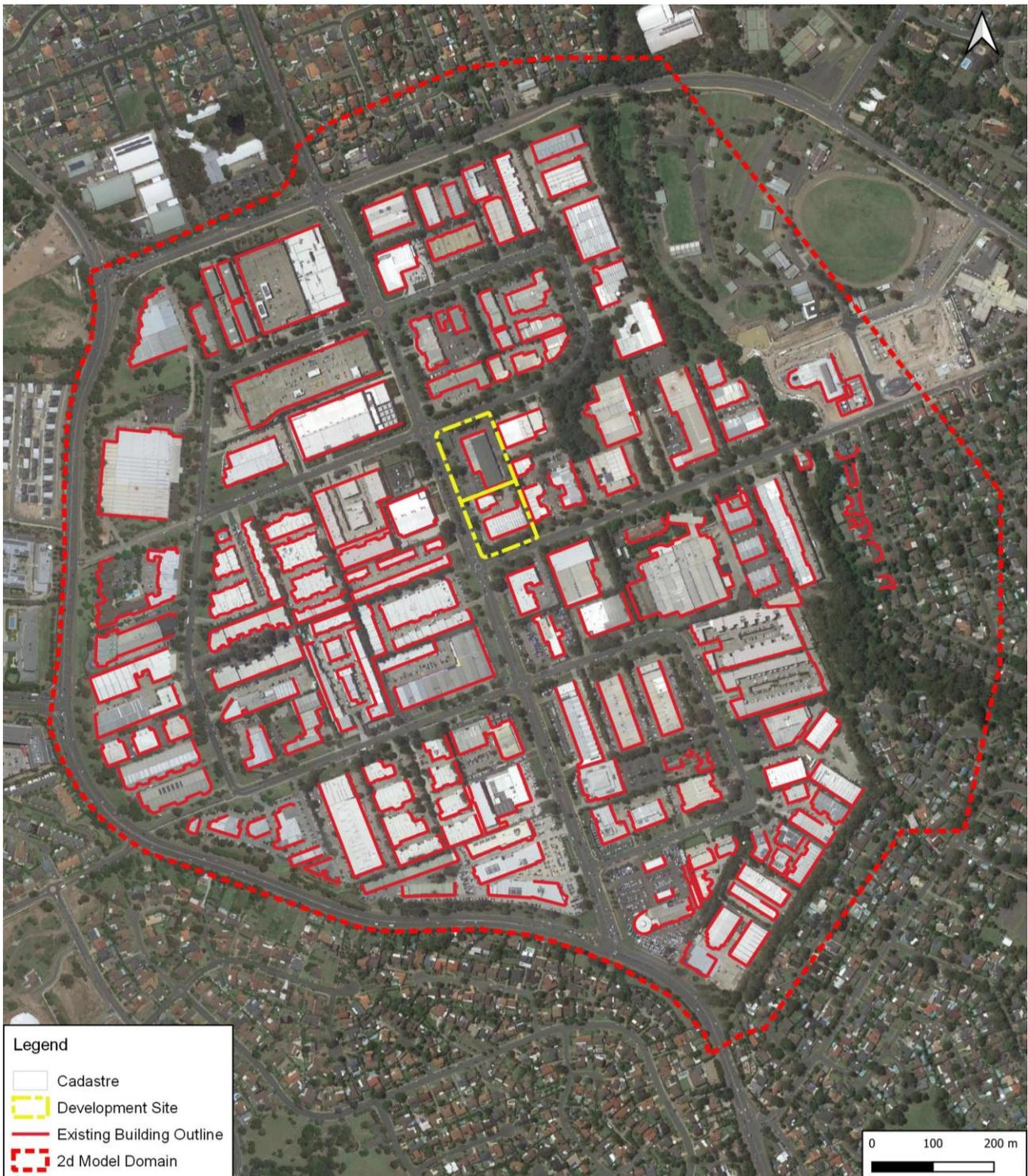
Figure 9 – Existing Building Outlines in TUFLOW Model
