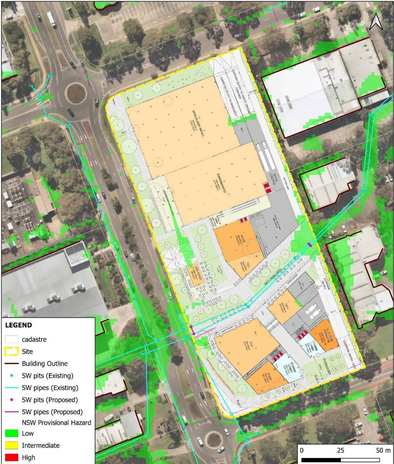
Figure 23 – NSW Provisional Flood Hazard (1%AEP) – Post Development Conditions – 2013 Tuflo Engine
