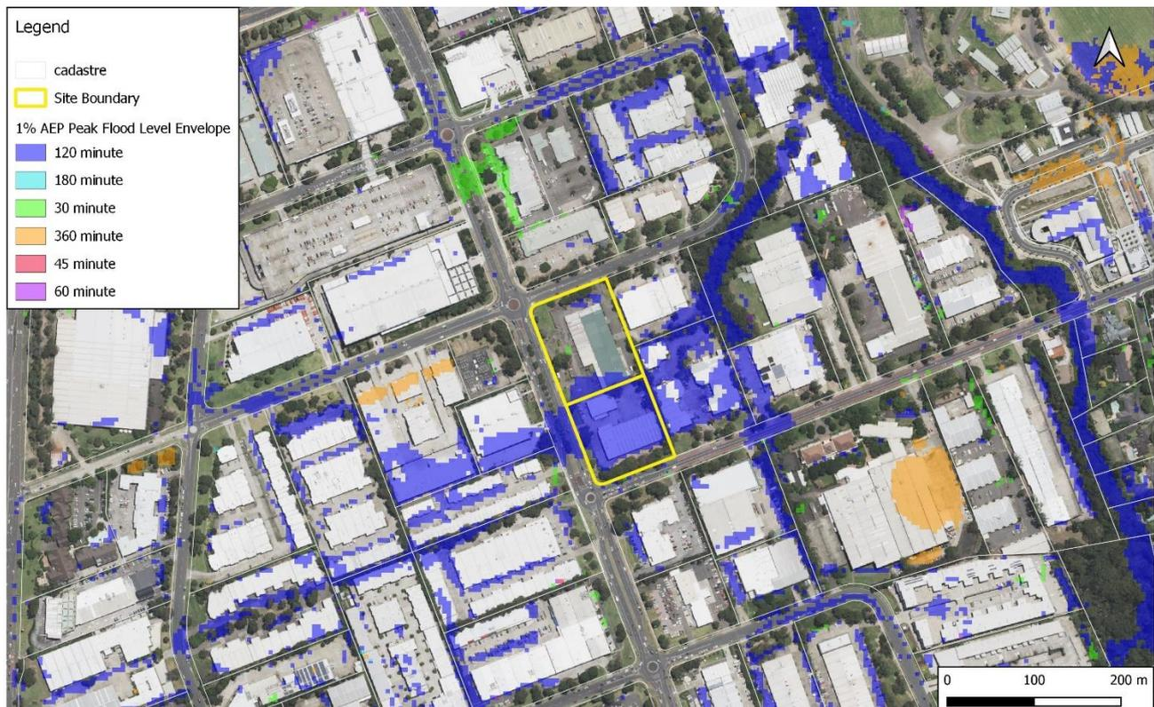
Figure 6 – 1% AEP Peak Flood Level - Envelope Results
